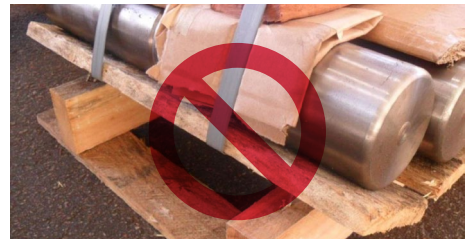
Figure 2: This is unsafe. Heavy roller pins have had restraints applied over the pallet top slats, and not the pallet under-bearers.
