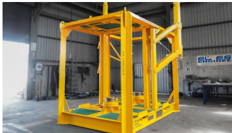
Figure 12: Transport Frame used for subsea equipment for the Greater Western Flank (GWF) Project
