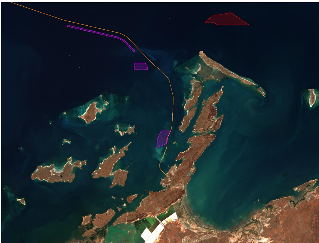
Figure 32: Satellite imagery captured from Sentinel-2 at 10:32 (local time) on 23 July 2023 (top image) and 22 August 2023 (bottom image) during trenching and spoil disposal activities. Trunkline is shown in orange, spoil grounds in purple and borrow ground in red
