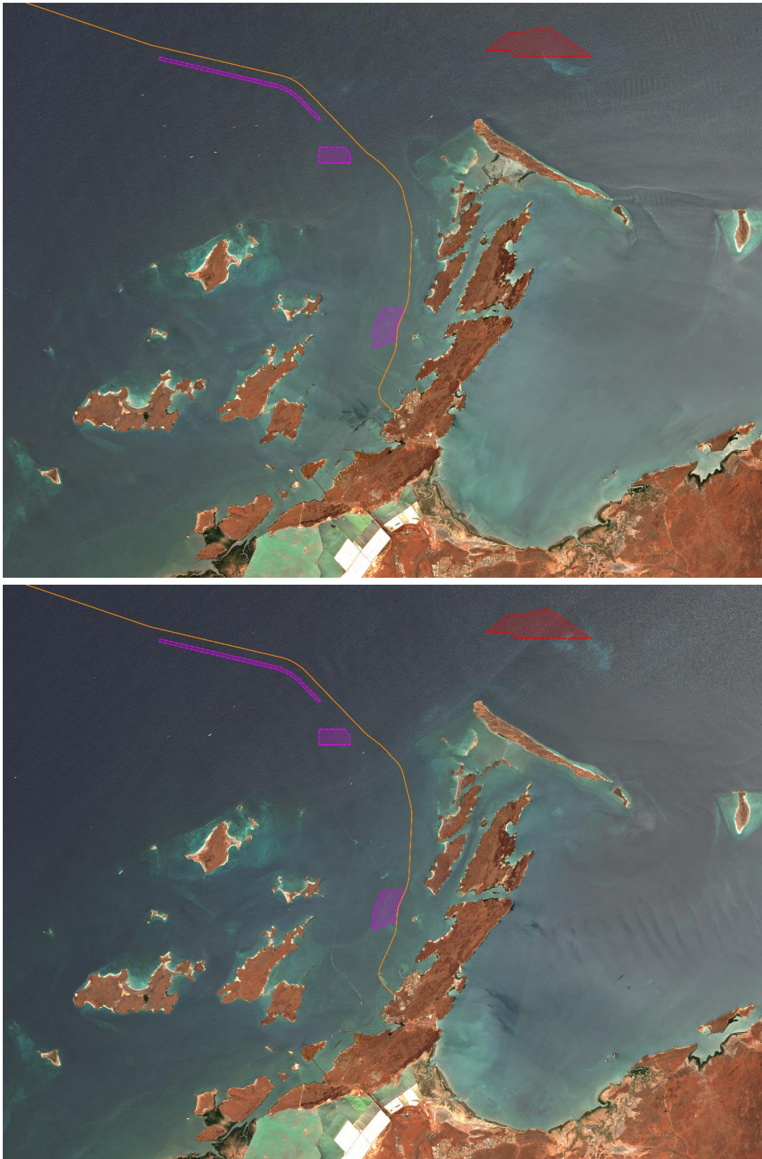
Figure 33: Satellite imagery captured from Sentinel-2 at 10:32 (local time) on 30 December 2023 (top image) and 9 January 2024 (bottom image), with visible plumes during borrow ground dredging. Trunkline is shown in orange, spoil grounds in purple and borrow ground in red
