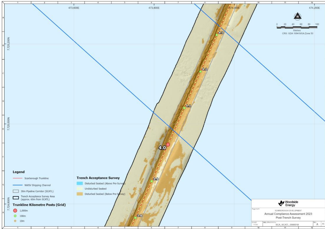
Figure 5-6 Example 5: Post-trenching survey along the trunkline corridor 2 .
