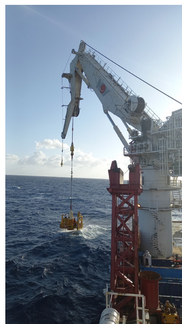
Typical subsea equipment recovery activity
