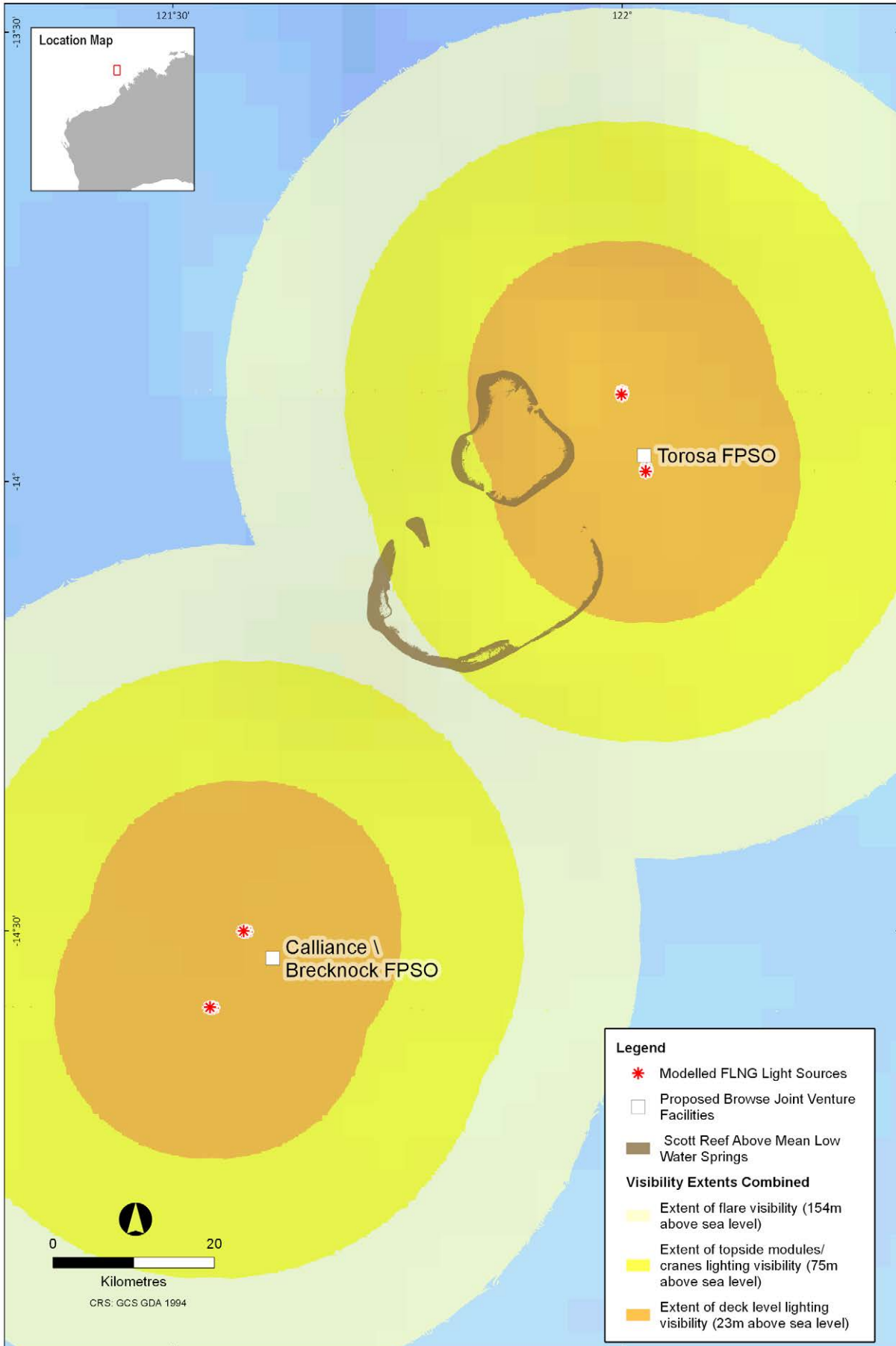
Figure 6-6 Line of sight assessment for previously proposed FLNG facilities locations at Torosa (refer to proposed Torosa FPSO), Brecknock and Calliance FPSO (Jacobs and SKM, 2014)
