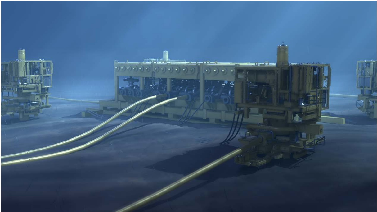
Figure 3-1 Indicative Layout of Subsea Infrastructure
